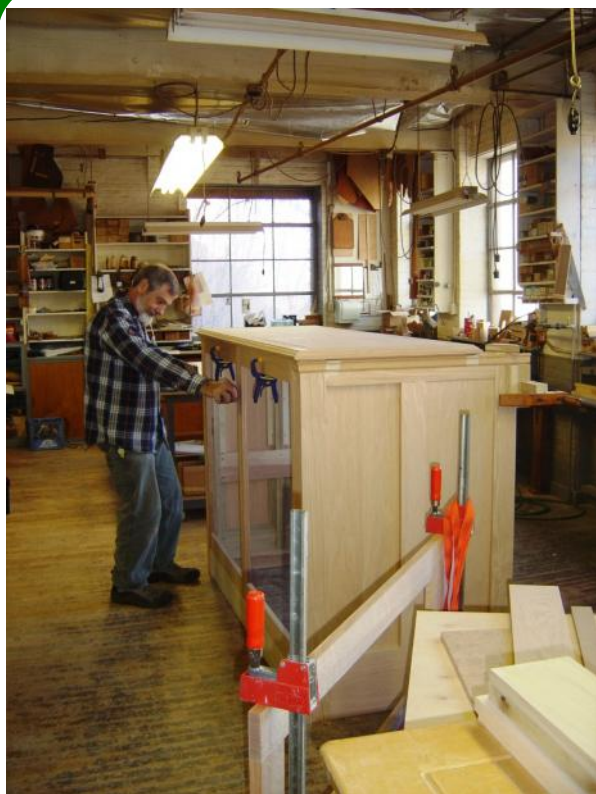
Above, cabinetmaker Robert Ferraro begins the dry-fit process of the new console for St. Edward's.
